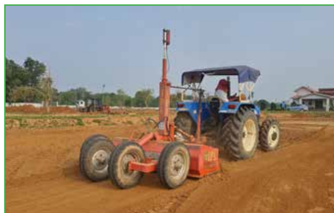
Land levelling using laser technology
