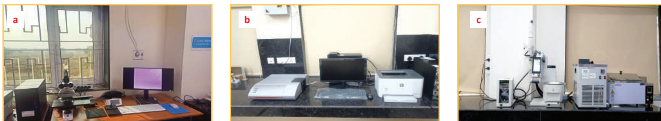
Figure 24. Instrumentation facilities procured and installed in the year, 2023 (a) Computer Assisted Semen Analyzer (b) Zeta Potential Analyzer and (c) Rotary evaporator
